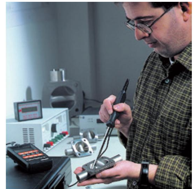
Delta Ferrite measurement of stainless steel valve bodies
