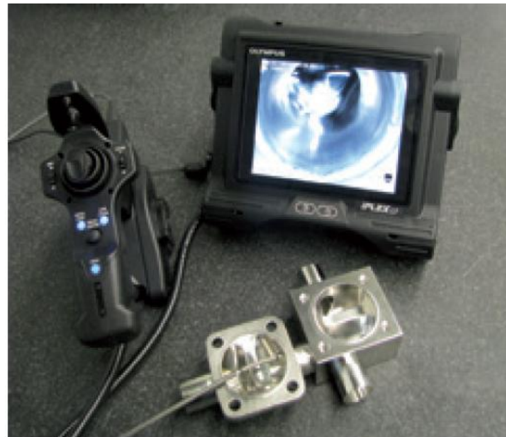
Borescope inspection of the interior surface and weld seams of valves for aseptic applications
