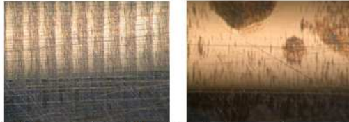
Images of stainless steel piston after use
