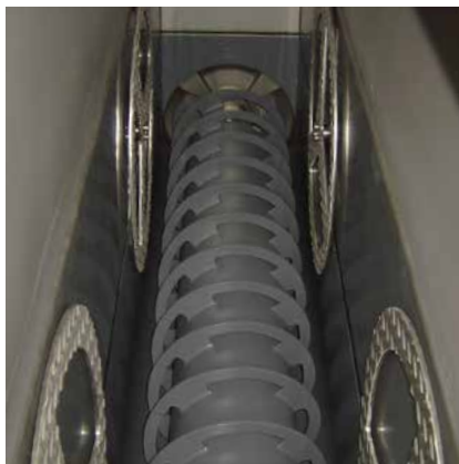
Internal view of the progressing cavity pump: Attachment with aBP-Module® to prevent bridging
