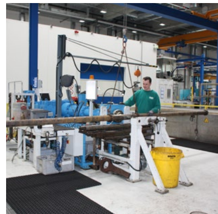
Extruder with stator for conveying oil
