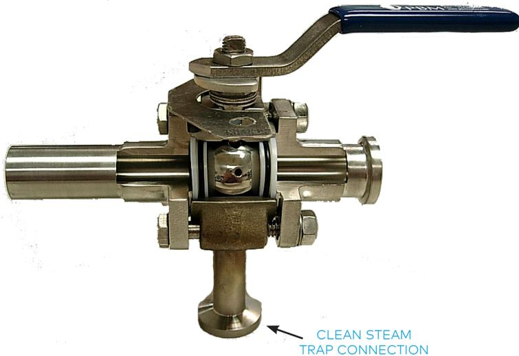
The 2-Way Sanitary Steam Trap valves use body purge port and ball purge holes to direct flow to the trap while shutting off flow downstream. Permits sampling of steam for purity and safely isolates trap for ease of maintenance.
