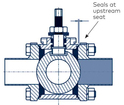
Valve body bolts compress valve seats against the ball, providing bidirectional sealing at the upstream seat. To compensate for seat wear, body bolts can be slightly tightened to re-compress seats against ball.
