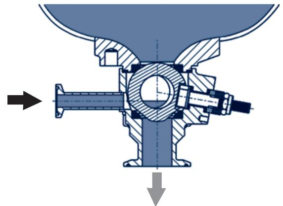
This means on valves mounted vertically like IMI PBM's Angle Stem Flush Tank valve, the valve seals on the upstream seat, thus allowing the body to be purged and drained without process interruption.
