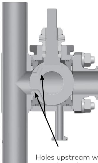
Holes upstream will allow run side to drain.
