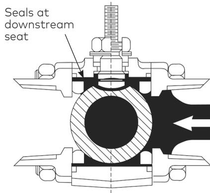
Line pressure pushes ball downstream in the ball-closed position, providing sealing at the downstream seat. There is no adjustment to compensate for seat wear.
