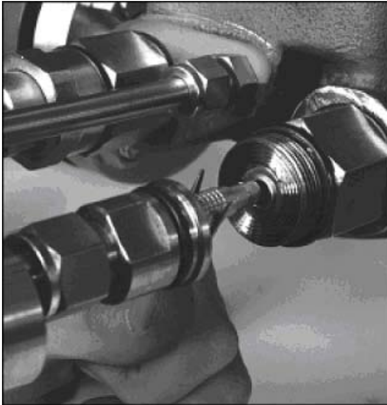
Figure 10: Disconnecting Lemo™ Connector
