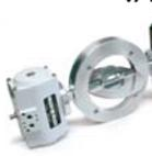
The **DOUBLE VALVE** is composed by a butterfly with a small concentric inside rotor. The butterfly transfers a big quantity of product and the rotor allows to reach the required quantity, with the precision of  $\pm 0 - 20$  gr. detected by an apposite weighing system.
