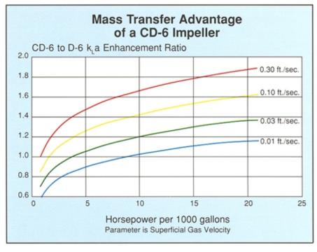
ratio of k<sub>L</sub>a for a CD-6 impeller to a flat-blade disc (D-6) impeller are shown in the graph as a function of horsepower per one thousand gallons and superficial gas velocity.
