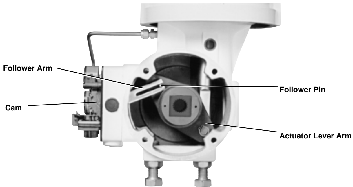
Figure 8: Beta Positioner Installation on Rotary Actuator
